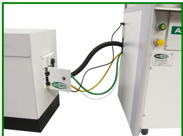
Docking station on LHS of fume cupboard
