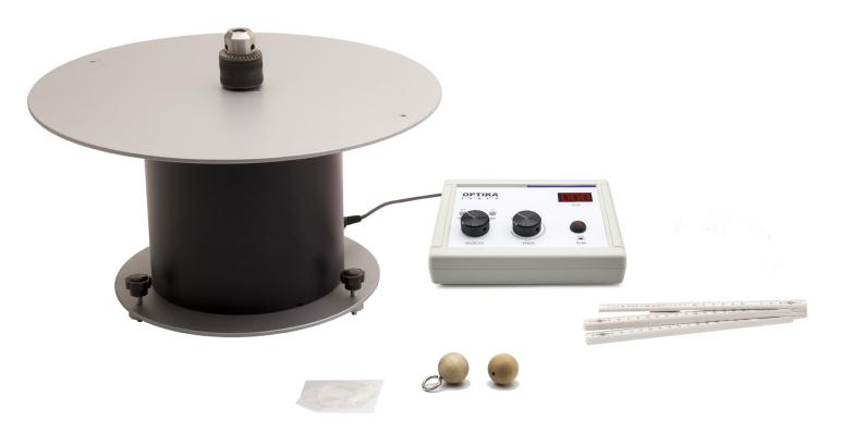
Optika rotating platform allows students not only to verify the relations between the fundamental quantities which characterize rotational motion, but also to perform experiments on an important topic: inertial and non-inertial systems.
