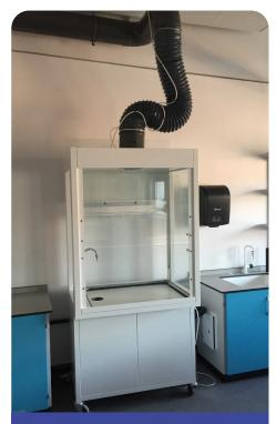
The fume cupboard can be moved up to 2m before being locked into position using a docking station
