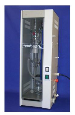
The Calypso can be connected directly to a mains tap supply or where preferred, from a pre-treated water supply using the optional pre-treated feed kit. An automatic flow controller governs the rate of water consumption and allows the unit to be used over a wide tap water pressure range. In the pre-treated mode, purified water is fed directly to the boiler and tap water is used for cooling purposes only.
