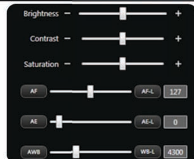
Advanced SLR Style Camera Controls: Adjust the image, including Focus, Exposure and White Balance
