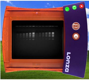
5.2.2 When you turn the light on, the camera will automatically adjust its exposure settings to show an optimized image. You will then be able to monitor the separation of fragments during the course of the experiment.
