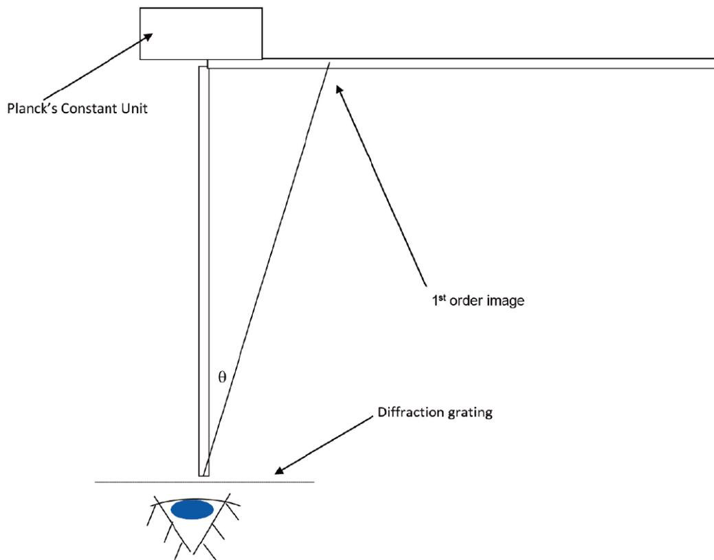
Using the diffraction grating, view the LEDs from the end of the metre rule as shown
