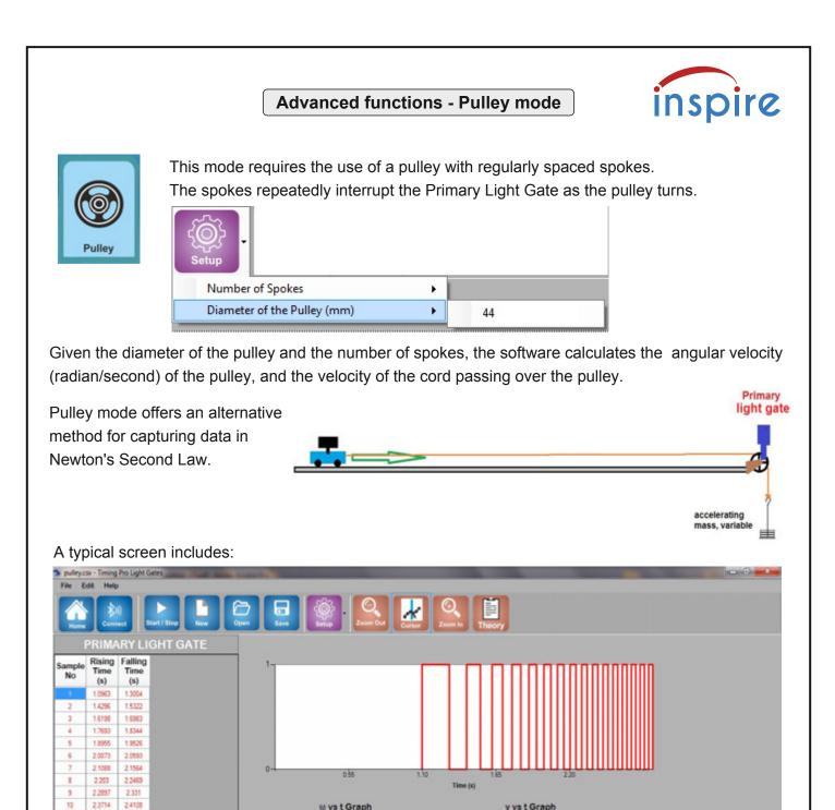
the data table recording every interruption of the light gate, the event graph clearly indicating whether the pulley and cord were accelerating, graphs of angular velocity and velocity against time, the summary chart of calculated values for angular and linear velocity.
