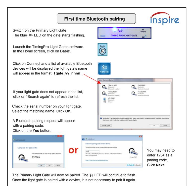
In future, after launching TimingPro software, click on Connect to establish communication between the software and a light gate that has already been paired.
