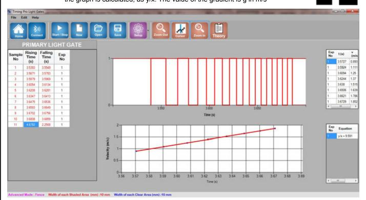
Clicking on New will clear the results. Clicking on Start, **without** clicking New, allows for results to be added to the data tables and overlaid in the graph. New data is identified as Exp No 2, Exp No 3 etc. Zoom in and the Cursor provide tools for exploring the data in detail.
