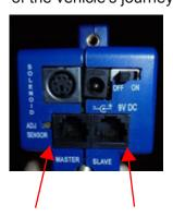
The Primary Light Gate has two sockets which will accept the link wire to Secondary light gates. These are marked MASTER and SLAVE.
