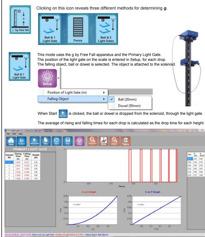
For each drop, which can be from a range of heights entered via Setup, the software calculates a value of g. A point is added to the graphs of h vs t and h vs t<sup>2</sup> The coefficient of t<sup>2</sup> in h vs t is ½ g and the gradient of the h vs t<sup>2</sup> graph is also 1/2 g. In the example above, that is 4.84, giving a value for g of 9.68 m/s<sup>2</sup>
