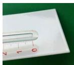
N.B. Before carrying out the experiment, ensure that the base of the air column in the capillary tube is aligned with the zero mark on the base plate. If there is a small amount of oil at the bottom of the tube, then set the top of that oil to the zero mark. This is to ensure that you are measuring the actual length of the trapped air.
