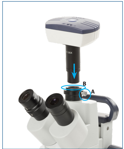
The EduBlue trinocular head. To adjust the height of the camera, loosen the screw (A), then turn the top part (B) up or down. Retighten the screw
