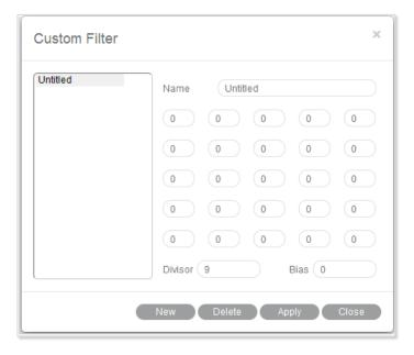
To define a new filter, click "New" and enter the name of the new filter. Enter values into the blanks to create a filter matrix with divisor and bias.
