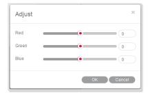
The three sliders are used to adjust the red, green and blue color channels of the active image. The value range always is from -100 to +100 with default value "0".
