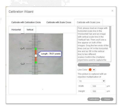
Click the Calibration button to continue as in Calibration with Calibration Circle.
