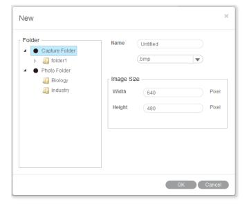
Select the format of the image file (jpg; bmp; tiff; png) and the file name. "png" is a proprietary Motic format which can only be opened with Motic Images Software. Define the image size. Capture Folder defines the location where the new image file should be saved.
