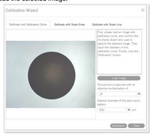
Select the magnification of the objective used for taking this picture, enter the diameter of the calibration dot (vacuum-metallized on the calibration slide) in the corresponding box. Click "**Calibration**" to continue. Check the x/y-axis values; they should only differ one decimal place. If not, the illumination is inappropriate.
