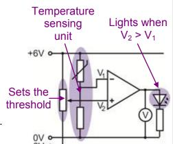
Near the switching threshold, any electrical noise could push the signal over the threshold, and cause the output to switch rapidly on and off, from the noise alone. Then, it may be better to use a Schmitt trigger circuit.
