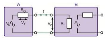
The diagram shows two subsystems,  $\bf A$  and  $\bf B$ . Our design aim is to pass on as much of the voltage  $V_S$  as possible. In other words, we want  $V_2$ , the voltage 'seen' by  $\bf B$ , to be as close as possible to  $V_S$ , the voltage generated by  $\bf A$ .
