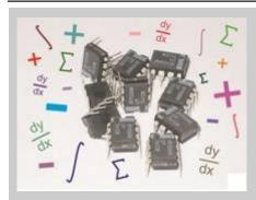
Operational amplifiers (op-amps) are used in a wide range of avionic applications. In fact, they are the most commonly used analogue IC, used in audio systems and instrumentation systems, used to perform mathematical operations, (hence their name) such as addition, subtraction, and integral and differential calculus. They were at the heart of analogue computing long before digital computers took over.
