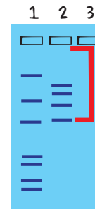
Figure 3: Measure distance migrated from the lower edge of the well to the lower edge of each band.
