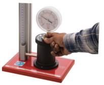
4. Tighten the screw on the valve.
