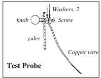
(2) <u>Neon Bulb Probe</u> Mount a small neon bulb (i.e. Ne<sub>2</sub>) on a plastic ruler. Turn the two lead wires at right angles, with one protruding from the ruler by 1 ". Solder an insulated copper wire to the other end and ground it by connecting it to the ground connection on the generator base.
