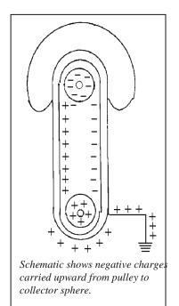
A similar comb (electrode) is provided at the upper end where it will provide a path for negative charges to be taken to the collector dome. The plastic pulley retains the positive charges that it acquired.
