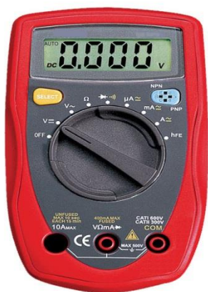
Multimeter set to read DC Volts
