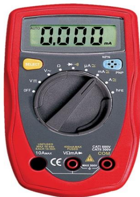
Multimeter set to read mA Current
